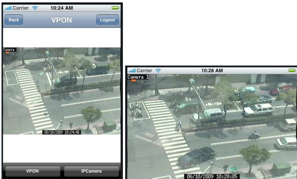
When you turn one channel full-screen, you can do PTZ control on it. (Of course, that means the camera you chose is a PTZ-control camera)
