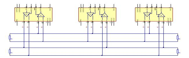
Example 2-wire network electrical connection: to enable 2-wire RS-485 configuration in Teltonika router, you need to connect D\_P to R\_P and D\_N to R\_N at the device RS-485 socket. Termination resistors are placed at each cable end.
