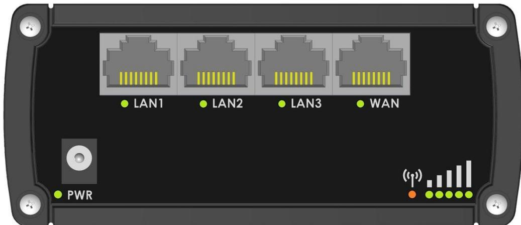
RUT9xx can be powered from power socket and over Ethernet simultaneously. Power socket has higher priority meaning that the device will draw power from power socket as long as it is available.
