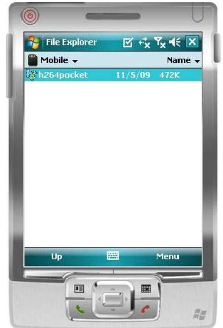
Step 2: Install the application software “**Jrviewer.CAB**” and “**H264Pocket.CAB**” in your mobile device, two folders named “**Jrviewer**” and “**H264Pocket**” will be created. It might be installed automatically after downloading; otherwise, select it from the downloading file for installation.
