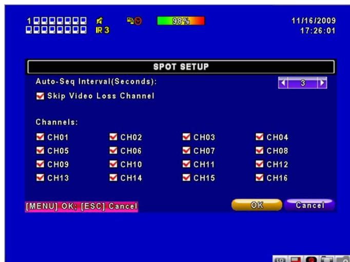
The DVR has two modes of video output; one is main video output, the other is spot video output. SPOT setup is for controlling the order of channels the system cycles through in SPOT mode. User can monitor every channel in the SPOT mode.
