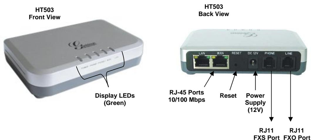
The HT503 has one FXS port and one FXO port. The PHONE port next to the power supply is an FXS port. The LINE port on the back right of the HT503 is an FXO port. Both the FXS port and the FXO port can have a separate SIP account. This is a key feature of HT503 as it supports simultaneous calls on both the FXS port and FXO port. Telephone calls can be originated from or terminated on the PSTN network remotely via the FXO port.
