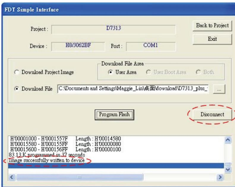
**STEP 7:** Power OFF the keyboard. The keyboard’s firmware upgrade is finished.
