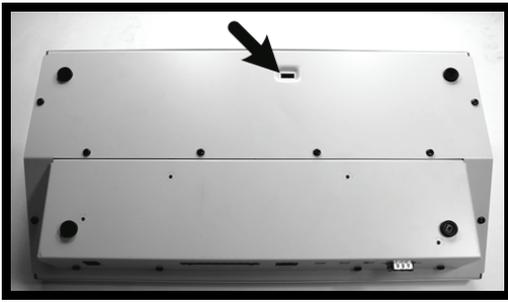
**STEP 2:** Connect the port COM1 or COM2 of the PC and keyboard with a RS-232 D-Sub9 cable (one-to-one, not a cross-over NULL-MODEM cable).
