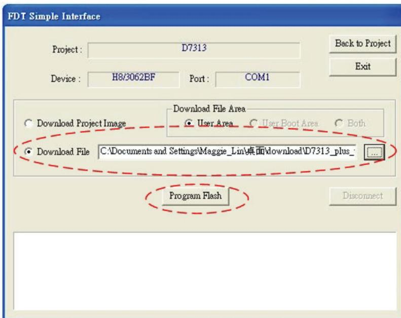
**STEP 4:** Click the “Program Flash” button to start upgrading firmware.
