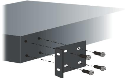
2. Then, install the VigorSwitch (with rack mount kit) on the 19-inch chassis by using other four screws.
