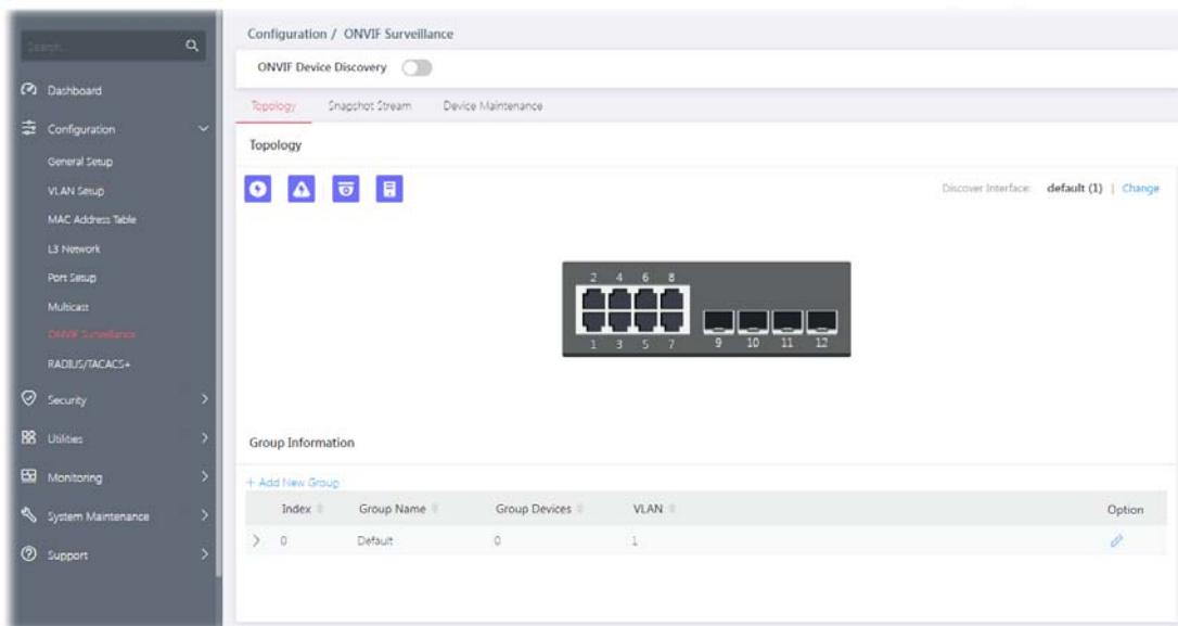
Switch the toggle to enable the **ONVIF Device Discovery** function. Then click **Apply**.
