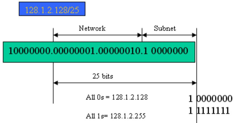
In this diagram, you can see the subnet mask with 25-bit long, 255.255.255.128, contains 126 members in the sub-netted network. Another is that the length of network prefix equals the number of the bit with 1s in that subnet mask. With this, you can easily count the number of IP addresses matched. The following table shows the result.
