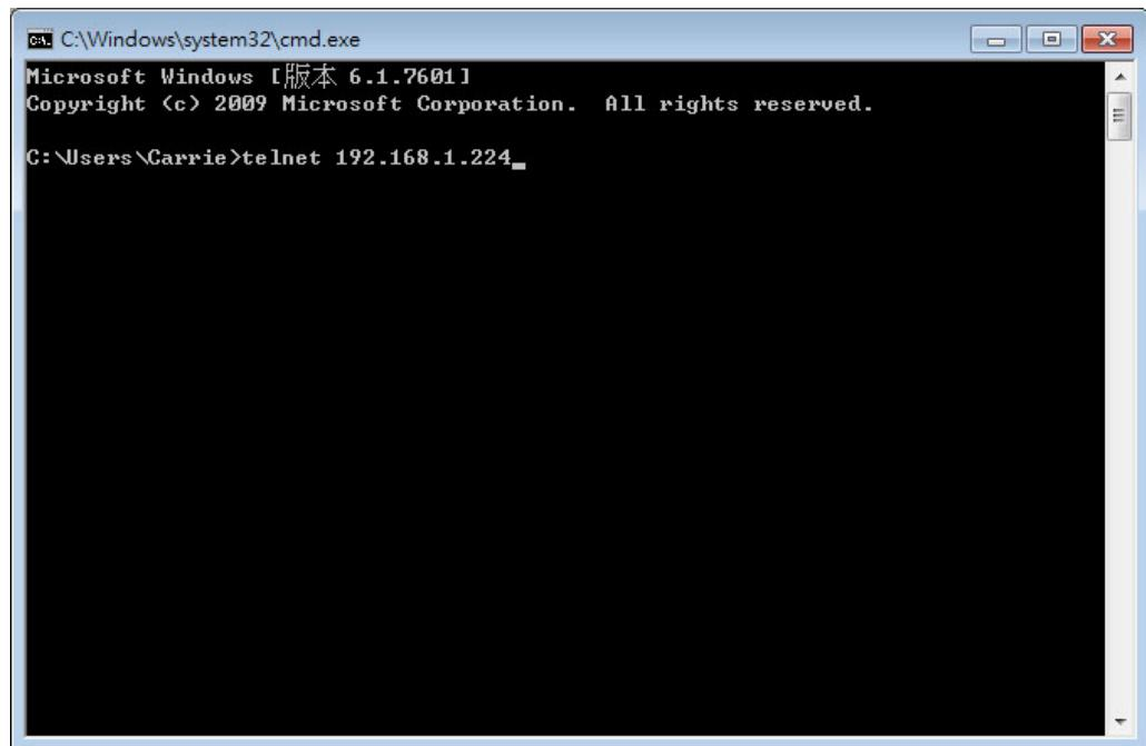
For users using previous Windows system (e.g., XP), simply click Start >> Run and type Telnet 192.168.1.224 in the Open box.
