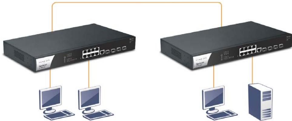
If VLAN is enabled and configured, each node in the network that can communicate each other directly is bounded in the same VLAN area.
