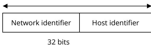
With the classful addressing, it divides IP address into three classes, class A, class B and class C. The rest of IP addresses are for multicast and broadcast. The bit length of the network prefix is the same as that of the subnet mask and is denoted as IP address/X, for example, 192.168.1.0/24. Each class has its address range described below.
