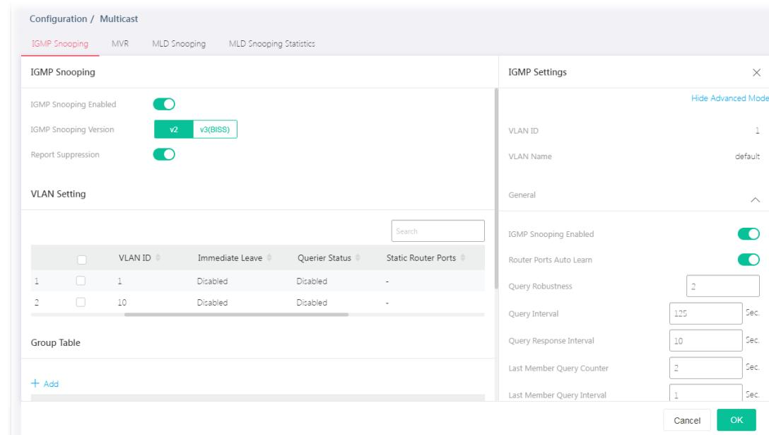
The screenshot shows the 'Configuration / Multicast' section with the 'IGMP Snooping' tab selected. On the left, there's a 'VLAN Setting' table for VLAN 1 and VLAN 10. On the right, an 'IGMP Settings' dialog box is open for VLAN 1. The dialog includes fields for 'VLAN ID' (1), 'VLAN Name' (default), and various configuration options like 'IGMP Snooping Enabled' (enabled), 'Router Ports Auto Learn' (enabled), and timers for 'Query Interval' (125 sec), 'Query Response Interval' (10 sec), etc.
