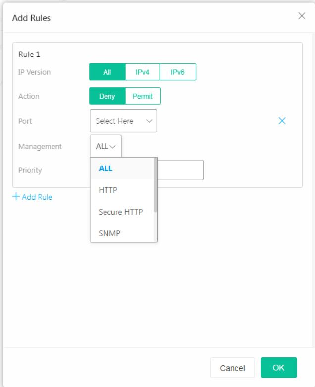
**IP Version** - Specify the IP address/subnet to which the ACL should be applied.
