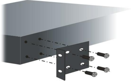
2. After the bracket installation, the VigorSwitch's chassis can be installed in a rack by using four screws for each side of the rack.
