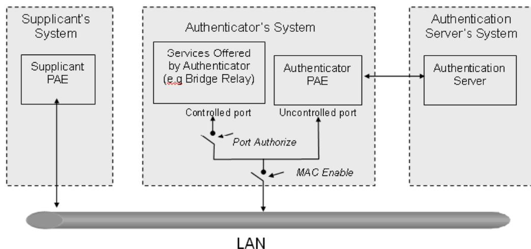
**Supplicant:** It is an entity being authenticated by an authenticator. It is used to communicate with the Authenticator PAE (Port Access Entity) by exchanging the authentication message when the Authenticator PAE request to it.
