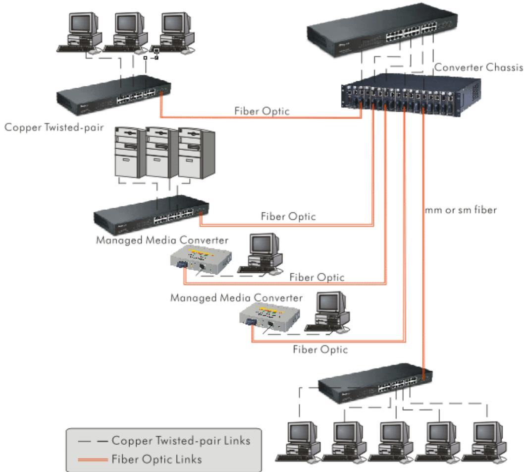
It is a system wide basic reference connection diagram. This diagram demonstrates how the switch and the various devices form the network infrastructure in a large-scale network.
