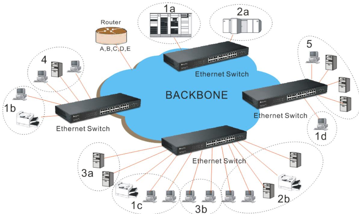
Now we apply VLAN technology to configure the system shown as the figure above. We can partition the users into the different logical networks which have their own broadcast domain. The traffic will not disturb among these logical networks. The users 1x (x denotes a ~ d) are members of VLAN 1. Any traffic within VLAN 1 does not flow to VLAN 2 and
