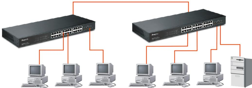
If VLAN is enabled and configured, each node in the network that can communicate each other directly is bounded in the same VLAN area.
