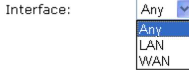
For example, the **Direction** setting in **Edit Filter Rule** will ask you specify IP or IP range for WAN or LAN or any IP address. If you choose LAN as the **Interface** here, and choose LAN as the direction setting in **Edit Filter Rule**, then all the IP addresses specified with LAN interface will be opened for you to choose in **Edit Filter Rule** page.
