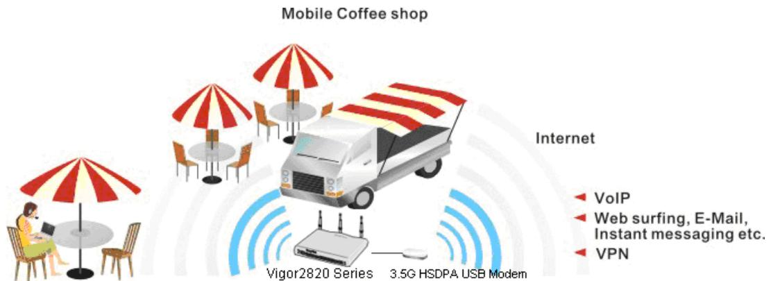
After connecting into the router, 3G USB Modem will be regarded as the second WAN port. However, the original Ethernet WAN1 still can be used and Load-Balance can be done in the router. Besides, 3G USB Modem in WAN2 also can be used as backup device. Therefore, when WAN1 is not available, the router will use 3.5G for supporting automatically. The supported 3G USB Modem will be listed on Draytek web site. Please visit [www.draytek.com](http://www.draytek.com) for more detailed information.
