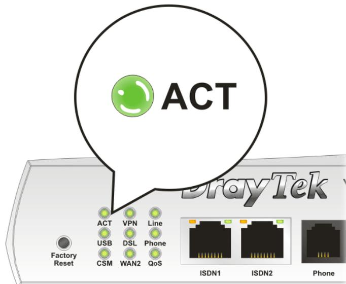
3. If not, it means that there is something wrong with the hardware status. Simply back to “**1.3 Hardware Installation**” to execute the hardware installation again. And then, try again.
