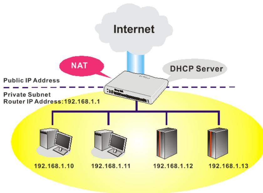
In some special case, you may have a public IP subnet from your ISP such as 220.135.240.0/24. This means that you can set up a public subnet or call second subnet that each host is equipped with a public IP address. As a part of the public subnet, the Vigor router will serve for IP routing to help hosts in the public subnet to communicate with other public hosts or servers outside. Therefore, the router should be set as the gateway for public hosts.
