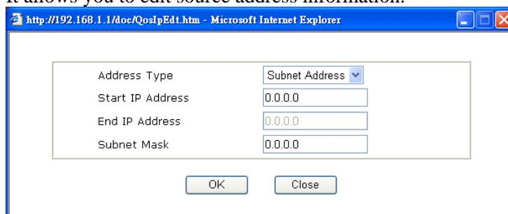
**Address Type** – Determine the address type for the source address.
