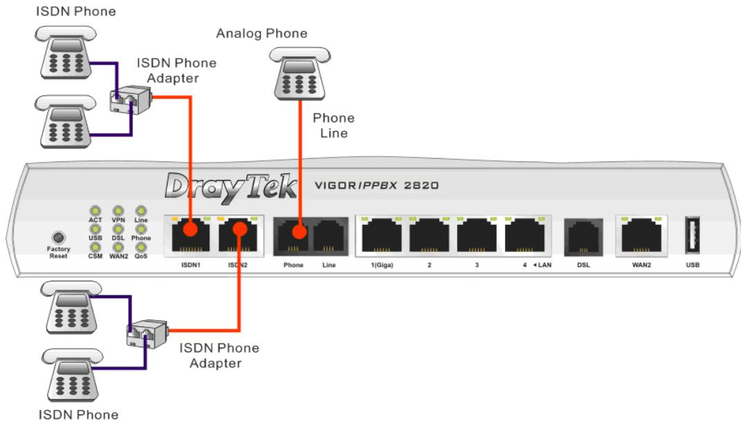
Yet, if the user configures ISDN port as TE Mode in **IP PBX>>PBX System>>Phone Settings**, the **green** LED will light on to indicate **ISDN-TE** is selected. Then, the port is specified for ISDN line only. Refer to the following figure for reference.
