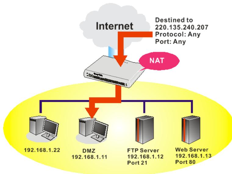
The inherent security properties of NAT are somewhat bypassed if you set up DMZ host. We suggest you to add additional filter rules or a secondary firewall.
