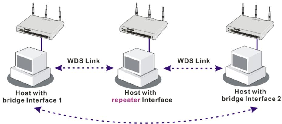
The major difference between these two modes is that: while in **Repeater** mode, the packets received from one peer AP can be repeated to another peer AP through WDS links. Yet in **Bridge** mode, packets received from a WDS link will only be forwarded to local wired or wireless hosts. In other words, only Repeater mode can do WDS-to-WDS packet forwarding.
