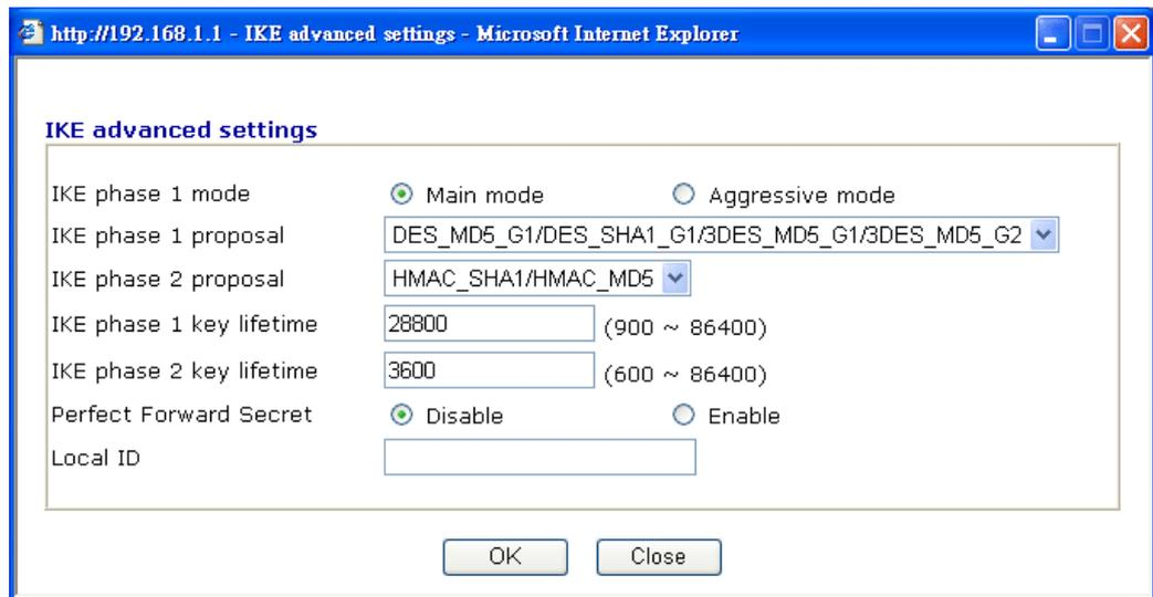
**IKE phase 1 mode** -Select from **Main** mode and **Aggressive** mode. The ultimate outcome is to exchange security proposals to create a protected secure channel. **Main** mode is more secure than **Aggressive** mode since more exchanges are done in a secure channel to set up the IPSec session. However, the **Aggressive** mode is faster. The default value in Vigor router is Main mode.
