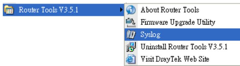
3. From the Syslog screen, select the router you want to monitor. Be reminded that in **Network Information**, select the network adapter used to connect to the router. Otherwise, you won’t succeed in retrieving information from the router.
