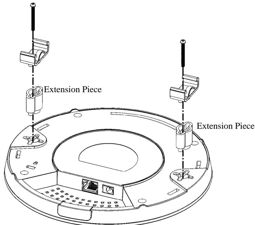
4. Use the T-Rail brackets to fasten the device on Light-weighted Steel Frame.
