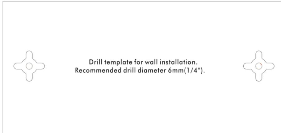
2. Place the template on the wall and drill the holes according to the recommended instruction.
