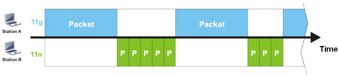
It is similar to automatic Bandwidth Limit. The dynamic bandwidth limit of each station depends on instant active station number and airtime assignment. Please note that Airtime Fairness of 2.4GHz and 5GHz are independent. But stations of different SSIDs function together, because they all use the same wireless channel. IN SPECIFIC ENVIRONMENTS, this function can reduce the bad influence of slow wireless devices and improve the overall wireless performance.
