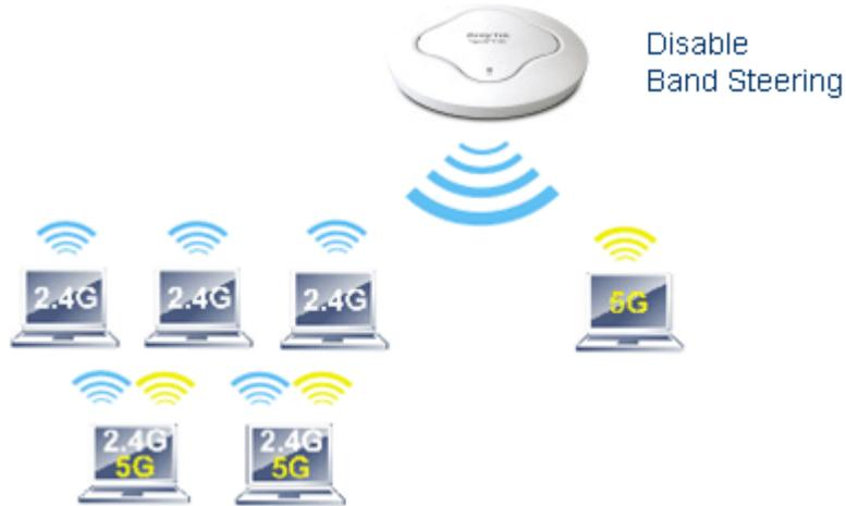
If dual-band is detected, the AP will let the wireless client connect to less congested wireless LAN, such as 5GHz to prevent from network congestion.
