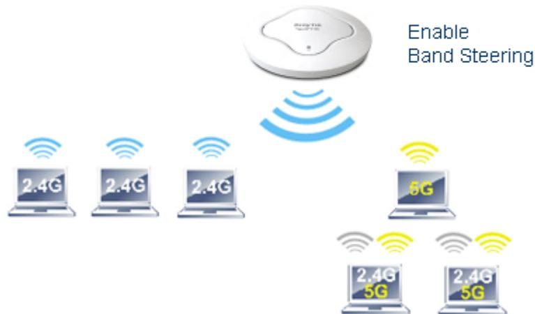
**Note:** To make Band Steering work successfully, SSID and security on 2.4GHz also MUST be broadcasted on 5GHz.
