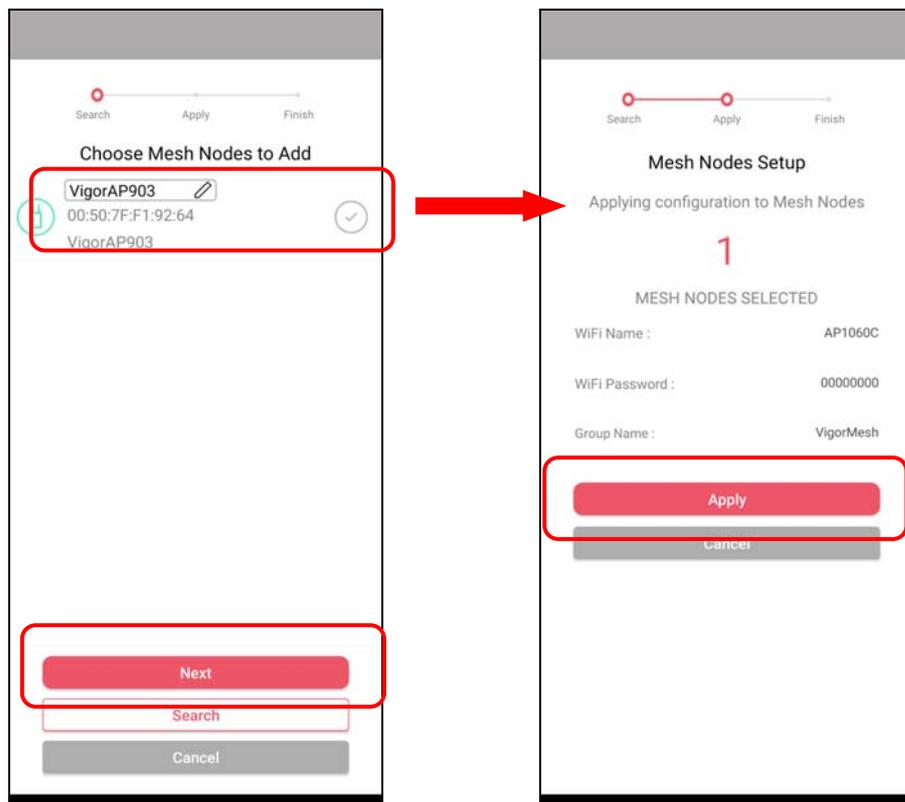
6. Wait until the mesh root applies general configuration to the mesh nodes. Later, current status of the mesh node(s) will be shown on the following page. Click **Finish**.
