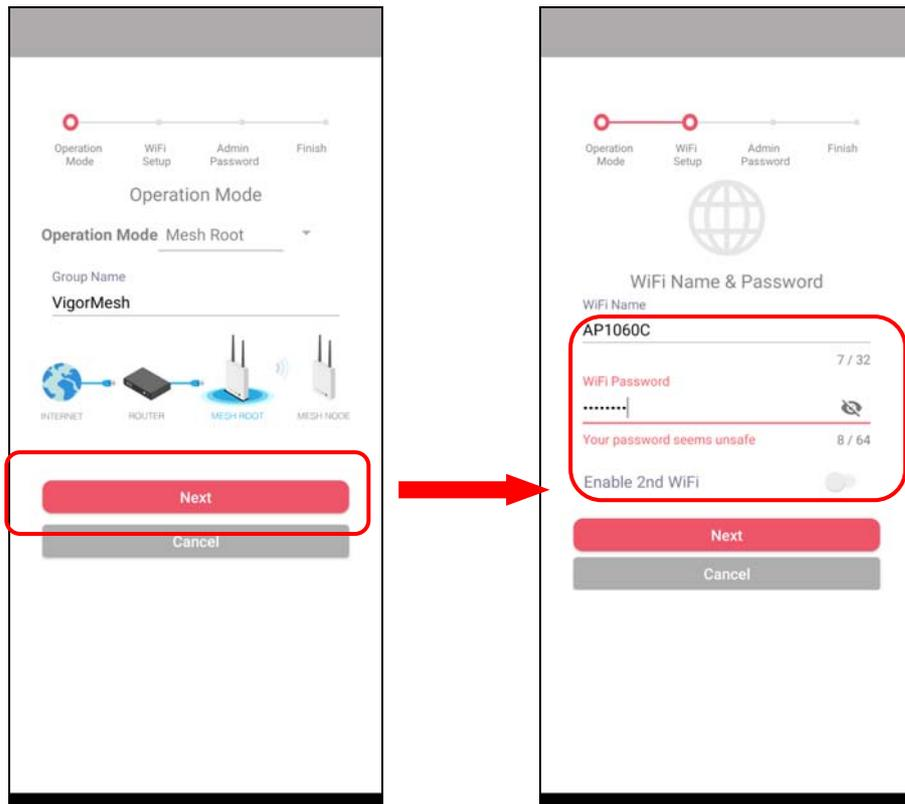
On the WiFi Name & Password page, enter the WiFi Name and the password (should be the same as the security settings set on the device's WUI). You can also enable 2nd SSID by enabling the function of 2nd WiFi. Then click the **Next** button.
