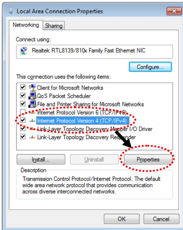
Under the General tab, click **Use the following IP address**. Then input the following settings in the respective field and click **OK** when finished.
