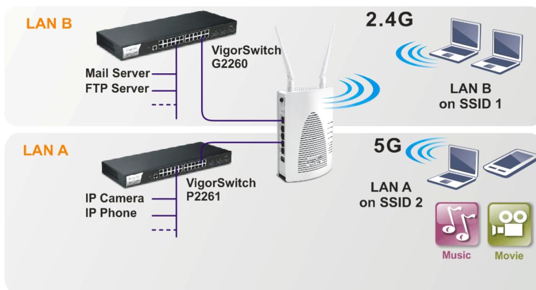
In the above figure, VigorAP 900 is used to control the wireless network connection. It can separate the wireless traffic between accessing internal server and the usage of video. Wireless station connecting to VigorAP 900 with SSID 2 can get the IP address with the network segment of 192.168.1.0/24 (LAN-A); wireless station connecting to VigorAP 900 with SSID 1 can get the IP address with the same network segment of 192.168.2.0/24 (LAN-B).
