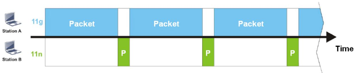
To improve this problem, Airtime Fairness is added for VigorAP900. Airtime Fairness function tries to assign *similar airtime* to each station (A/B) by controlling TX traffic. In the following figure, Station B(11n) has higher probability to send data packets than Station A(11g). By this way, Station B(fast rate) gets fair airtime and it's speed is not limited by Station A(slow rate).
