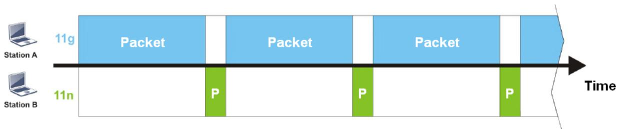
To improve this problem, Airtime Fairness is added for VigorAP900. Airtime Fairness function tries to assign *similar airtime* to each station (A/B) by controlling TX traffic. In the following figure, Station B(11n) has higher probability to send data packets than Station A(11g). By this way, Station B(fast rate) gets fair airtime and it's speed is not limited by Station A(slow rate).
