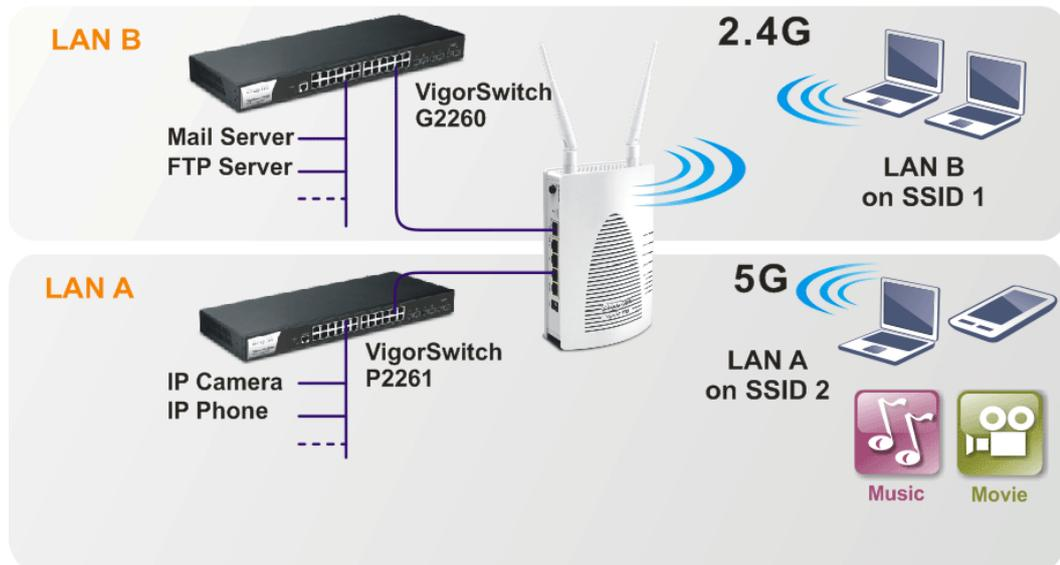
In the above figure, VigorAP 900 is used to control the wireless network connection. It can separate the wireless traffic between accessing internal server and the usage of video. Wireless station connecting to VigorAP 900 with SSID 2 can get the IP address with the network segment of 192.168.1.0/24 (LAN-A); wireless station connecting to VigorAP 900 with SSID 1 can get the IP address with the same network segment of 192.168.2.0/24 (LAN-B).
