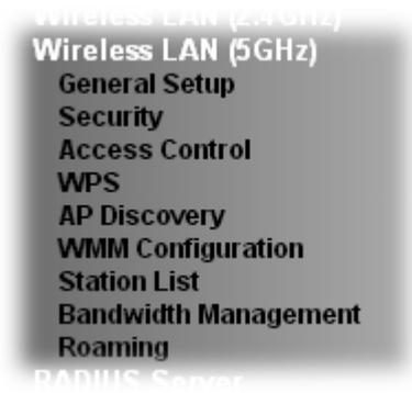
If no 5G dongle connected to VigorAP 900, an error message will be displayed and no function in this menu can be activated.
