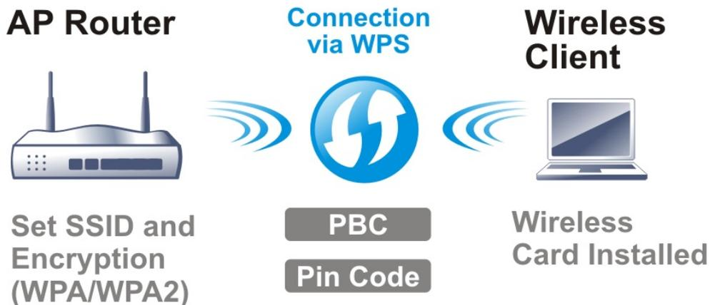
It is the simplest way to build connection between wireless network clients and VigorAP 1062C. Users do not need to select any encryption mode and type any long encryption passphrase to setup a
