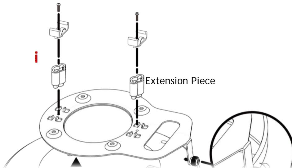
Attach the T-Rail brackets to the ceiling frame.
