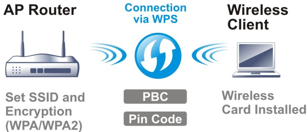
It is the simplest way to build connection between wireless network clients and VigorAP 1060C. Users do not need to select any encryption mode and type any long encryption passphrase to setup a wireless client every time. He/she only needs to press a button on wireless client, and WPS will connect for client and VigorAP 1060C automatically.
