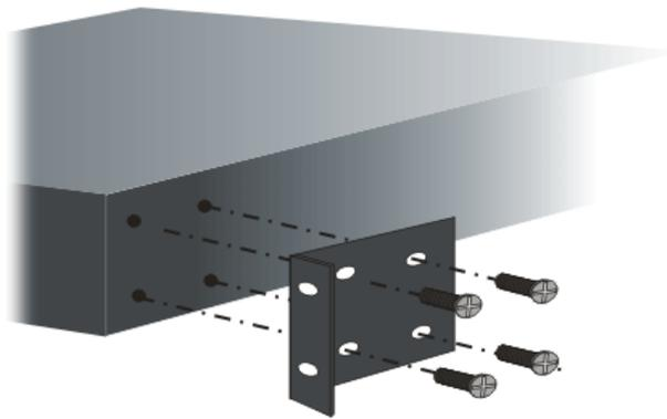
After the bracket installation, the Vigor3900 Series chassis can be installed in a rack by using four screws for each side of the rack.
