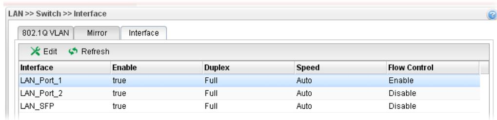
The screenshot shows a web-based configuration interface for a switch. The breadcrumb navigation at the top reads "LAN >> Switch >> Interface". Below this, there are three tabs: "802.1Q VLAN", "Mirror", and "Interface", with "Interface" being the active tab. Under the "Interface" tab, there are two buttons: "Edit" (with a green 'X' icon) and "Refresh" (with a circular arrow icon). Below the buttons is a table with the following data:
