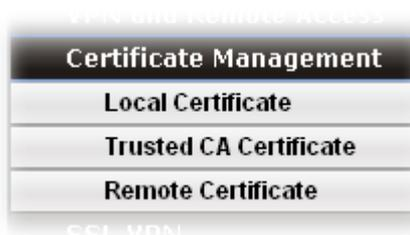
Local certificate is created by the end user and must be signed by a trusted CA center. Vigor3900 can serve as a trusted CA and is called with “Root CA”. Therefore, any user can ask for certificate signed by Vigor3900.
