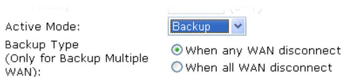
A screenshot of the 'Backup Type' configuration section. It shows a dropdown menu set to 'Backup'. Below it are two radio button options: 'When any WAN disconnect' (which is selected) and 'When all WAN disconnect'.
