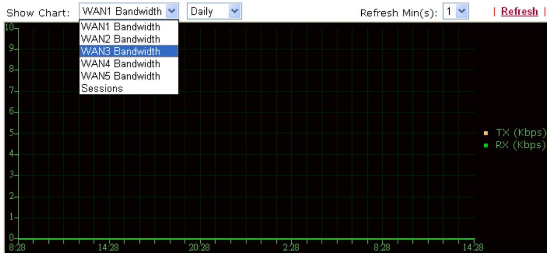
The horizontal axis represents time. Yet the vertical axis has different meanings. For WAN1/WAN2/WAN3/WAN4/WAN5 Bandwidth chart, the numbers displayed on vertical axis represent the numbers of the transmitted and received packets in the past.
