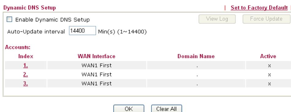
The screenshot shows the "Dynamic DNS Setup" configuration page. At the top right, there is a link "Set to Factory Default". Below the title, there is a checkbox "Enable Dynamic DNS Setup" and two buttons: "View Log" and "Force Update". The "Auto-Update interval" is set to "14400" with the unit "Min(s) (1~14400)". Below this is a table titled "Accounts:" with four columns: "Index", "WAN Interface", "Domain Name", and "Active".
