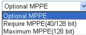
**Require MPPE (40/128bits)** - Selecting this option will force the router to encrypt packets by using the MPPE encryption algorithm. In addition, the remote dial-in user will use 40-bit to perform encryption prior to using 128-bit for encryption. In other words, if 128-bit MPPE encryption method is not available, then 40-bit encryption scheme will be applied to encrypt the data.
