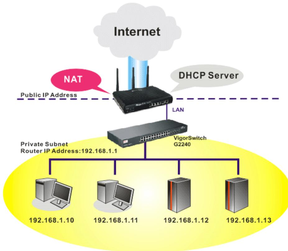
In some special case, you may have a public IP subnet from your ISP such as 220.135.240.0/24. This means that you can set up a public subnet or call second subnet that each host is equipped with a public IP address. As a part of the public subnet, the Vigor router will serve for IP routing to help hosts in the public subnet to communicate with other public hosts or servers outside. Therefore, the router should be set as the gateway for public hosts.
