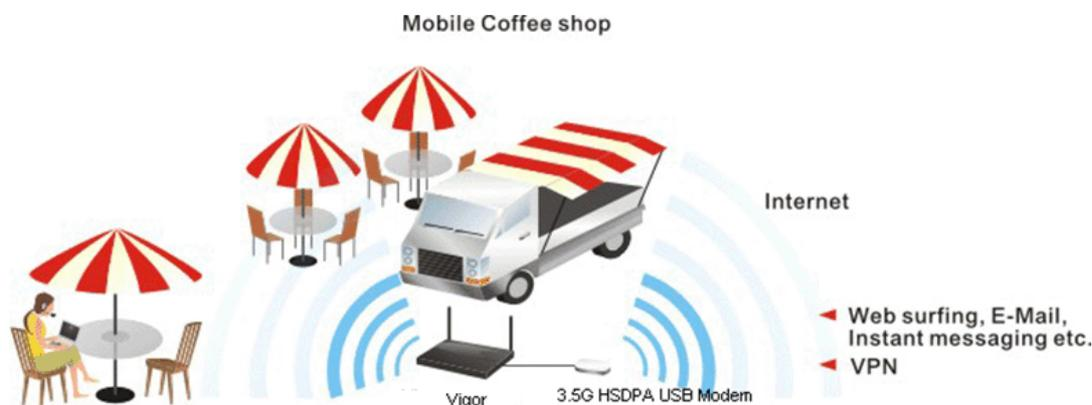
After connecting into the router, 3G USB Modem will be regarded as the fifth WAN port. However, the other Ethernet WAN ports still can be used and Load-Balance can be done in the router. Besides, 3G USB Modem in WAN5 also can be used as backup device. Therefore, when other Ethernet WAN port is not available, the router will use 3.5G for supporting
