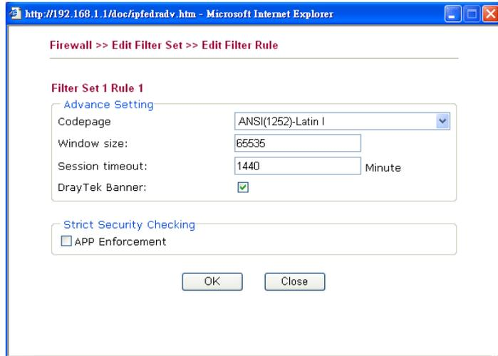
**Codepage** - This function is used to compare the characters among different languages. Choose correct codepage can help the system obtaining correct ASCII after decoding data from URL and enhance the correctness of URL Content Filter. The default value for this setting is ANSI 1252 Latin I. If you do not choose any codepage, no decoding job of URL will be processed. Please use the drop-down list to choose a codepage.
