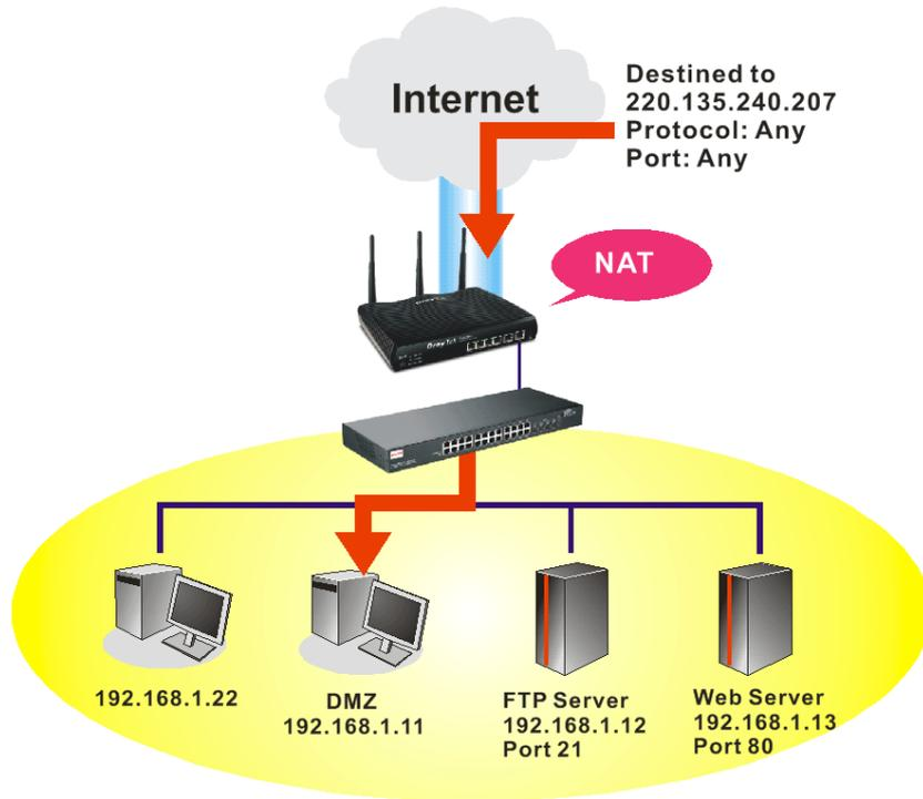
The security properties of NAT are somewhat bypassed if you set up DMZ host. We suggest you to add additional filter rules or a secondary firewall.
