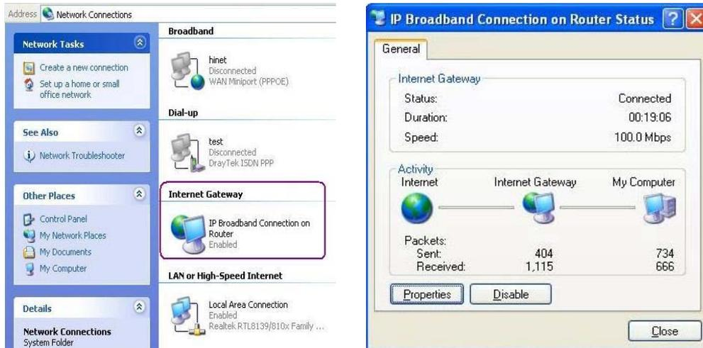
The UPnP facility on the router enables UPnP aware applications such as MSN Messenger to discover what are behind a NAT router. The application will also learn the external IP address and configure port mappings on the router. Subsequently, such a facility forwards packets from the external ports of the router to the internal ports used by the application.
