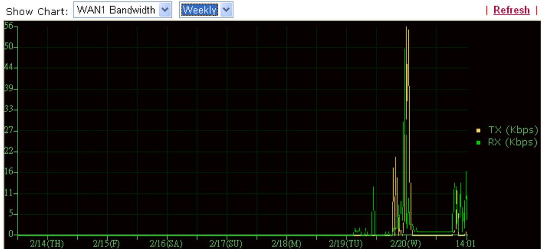
The horizontal axis represents time. Yet the vertical axis has different meanings. For WAN1/WAN2/WAN3/WAN4/WAN5 Bandwidth chart, the numbers displayed on vertical axis represent the numbers of the transmitted and received packets in the past.
