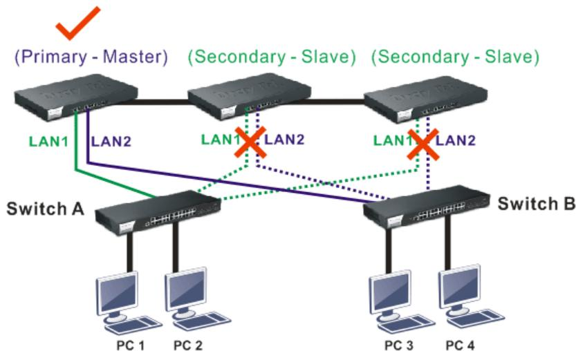
When the Master device fails, one of the slave devices will be chosen as the Master device to offer the network service for the connected PCs.
