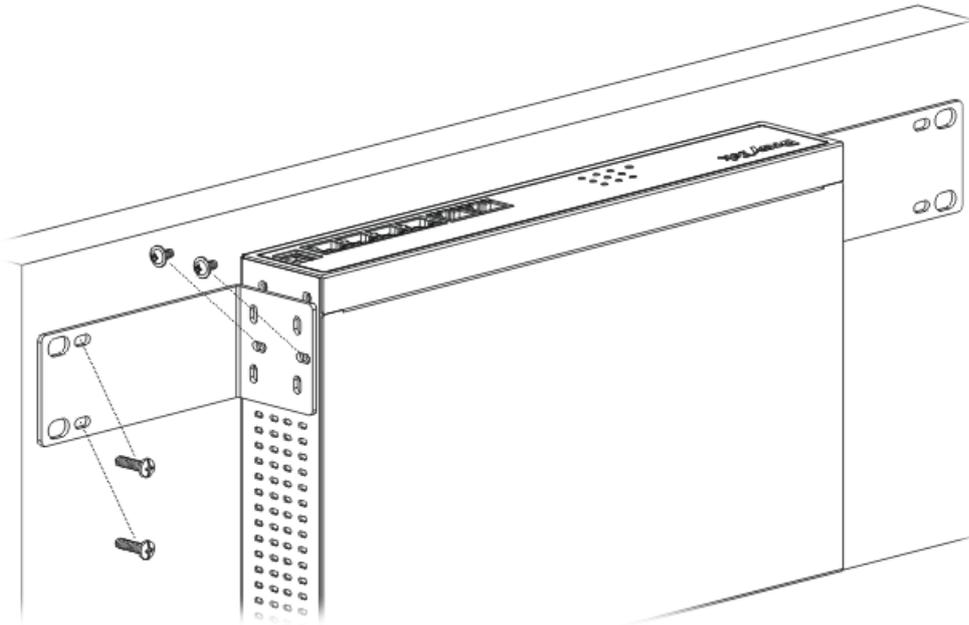
Then, continue to fasten the screws on the other side of the router and the wall with other screws.
