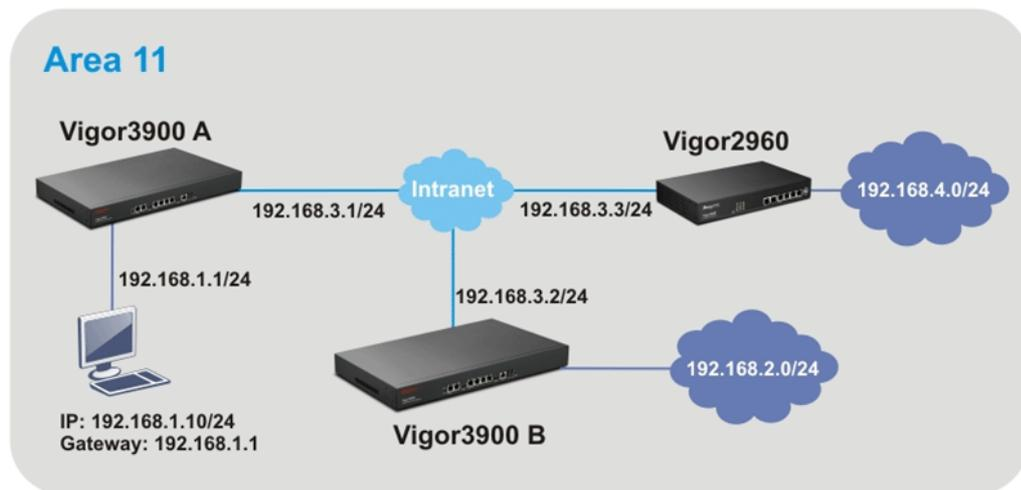
OSPF can place each router (e.g., Vigor3900A, Vigor3900B and Vigor2960 shown above) at the root of a tree and calculate the shortest path to each destination according to the cumulative cost to reach the destination.
