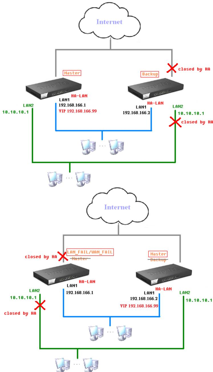
**Note:** Make sure the WAN interfaces for both Router A and Router B are well connected. Both routers can be used to access into Internet.
