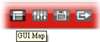
All the functions the router supports are listed with table clearly in this page. Users can click the function link to access into the setting page of the function for detailed configuration. Click the icon on the top of the main screen to display all the functions.
