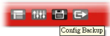
There is one way to store current used settings quickly by clicking the **Config Backup** icon. It allows you to backup current settings as a file. Such configuration file can be restored by using **System Maintenance>>Configuration Backup**.
