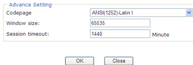
**Codepage** - This function is used to compare the characters among different languages. Choose correct codepage can help the system obtaining correct ASCII after decoding data from URL and enhance the correctness of URL Content Filter. The default value for this setting is ANSI 1252 Latin I. If you do not choose any codepage, no decoding job of URL will be processed. Please use the drop-down list to choose a codepage.
