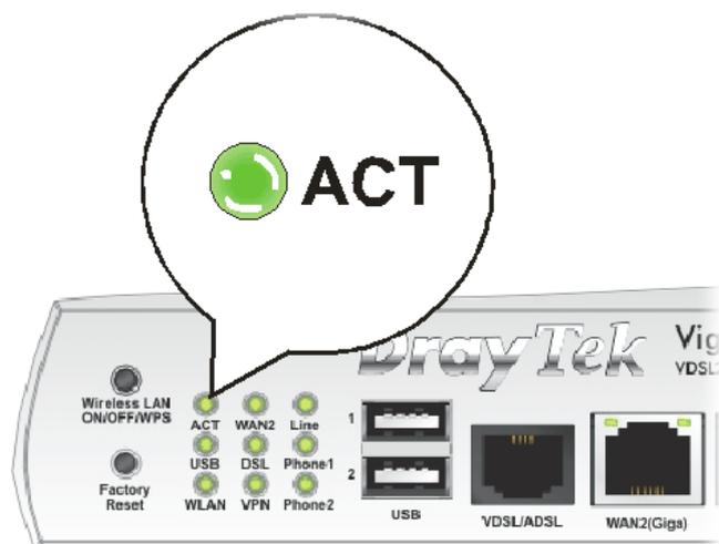
3. If not, it means that there is something wrong with the hardware status. Simply back to “**2.1 Hardware Installation**” to execute the hardware installation again. And then, try again.
