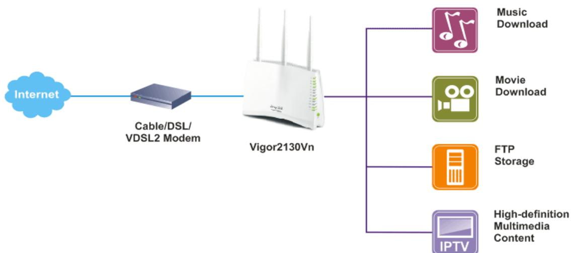
Vigor2130 supports up to 2 VPN tunnels using advanced protocols such as IPSec/PPTP (for remote dial-in only) with AES/3DES for encryption and MD5/SHA-1 for authentication.
