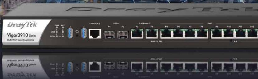
Vigor3910 is capable for bandwidth demanding network. The router features a powerful quad-core processor, eight WAN/LAN switchable interfaces, including two 10G SFP+ for fiber connectivity, two 2.5G Ethernet, RJ-45, and four Gigabit Ethernet, RJ-45. In addition, the router has four Gigabit Ethernet, RJ-45 as a fixed LAN interface.
