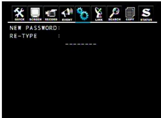
Insert your desired password and retype again using the CAMERA/ NUMBER INPUT buttons.
