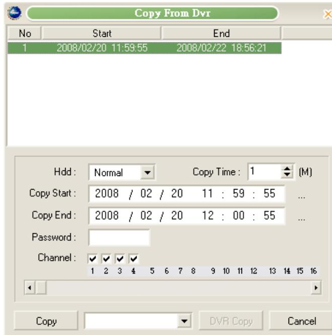
Select the desired HDD, Time and channel, click on “Copy” button to start copy. The Copying status will be shown as below. Click on “OK” button after the copy finished, the file will be saved in C:\Program Files\DVR \DVR-Viewer\COPY automatically.
