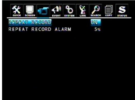
ON: When repeat recording, if the HDD is full, DVR will overwrite the recorded data automatically.
