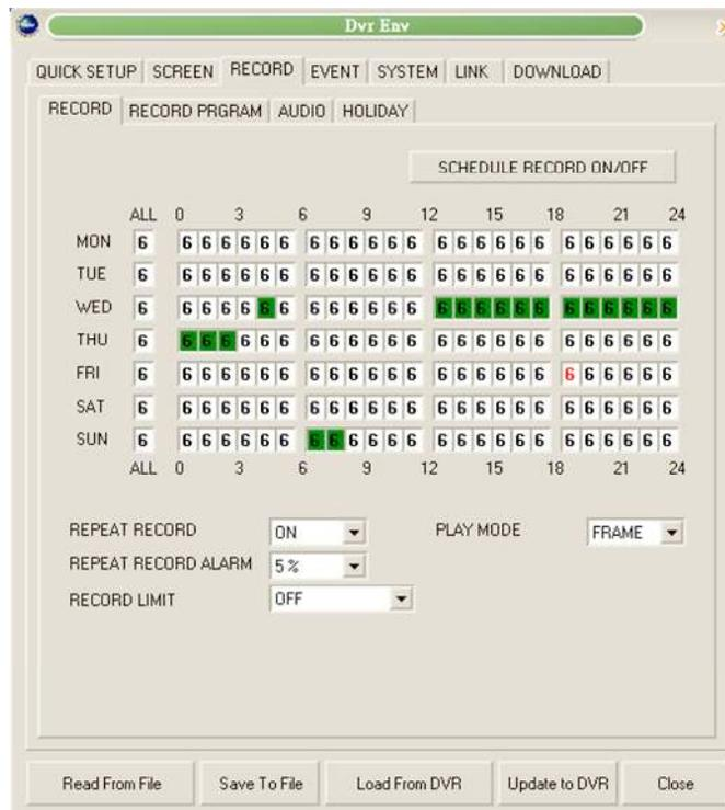
Turn the wheel scroll of the mouse on specific hour block to change the Record Program (0~9); double click the left key of mouse, the following window appears:
