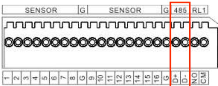
RS485 is use for connect to external device, such as keyboard or PTZ camera.
