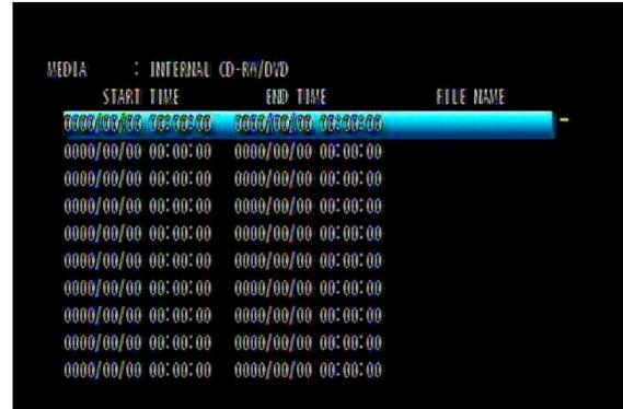
Select the desired storage device and press the ENTER button, the search results will be shown. Select the desired file and press ENTER to playback.
