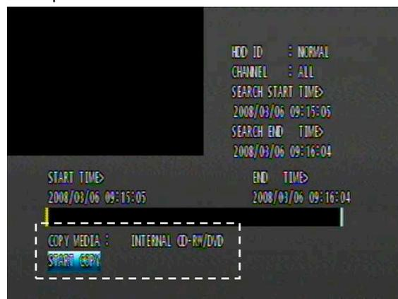
Make sure the record data was correct and select the storage device you want, then move the cursor to START COPY and press ENTER to copy.
