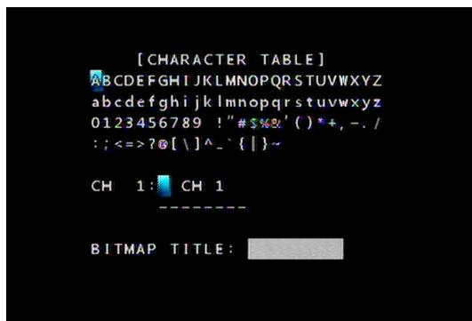
Select the character using the ▲, ▼, ◀, ▶ buttons and then press
