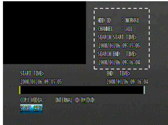
HDD ID: The HDD (HDD0, HDD1) which the record data saved. The default is NORMAL. The START TIME and END TIME of the selected record data will be shown on the screen. ◦
