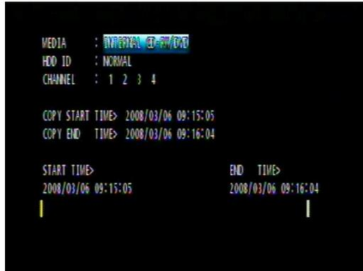
Select the desired MEDIA (INTERNAL CD-RW/DVD), HDD ID, CHANNEL, COPY START TIME, COPY END TIME and press the ENTER button to start the copy.
