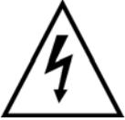
This symbol is intended to alert the user to the presence of unprotected “Dangerous voltage” within the product’s enclosure that may be strong enough to cause a risk of electric shock.
