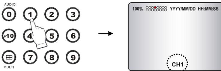
Press the desired camera number button to display on the monitor.
