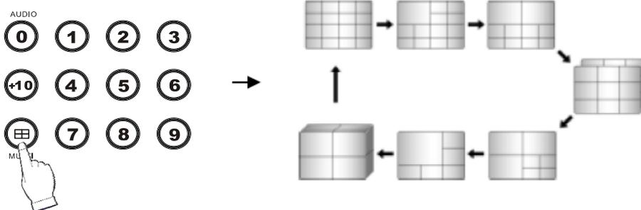
To change a single camera display to the multi camera, press the MULTI button.
