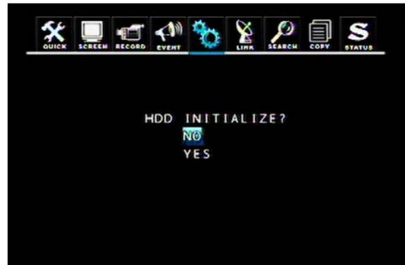
REC HDD INITIALIZE: Select YES and press ENTER button to format the HDD.
