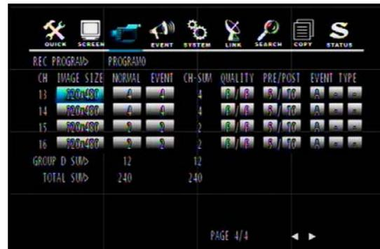
Four channels are grouped and placed in one page. The resolution is revealed in groups, which means, each group consists of four channels have the same types of resolution. Other setting can be selected by each camera. Move down to change to the next page or move cursor to the bottom of screen in order to click the arrows.
