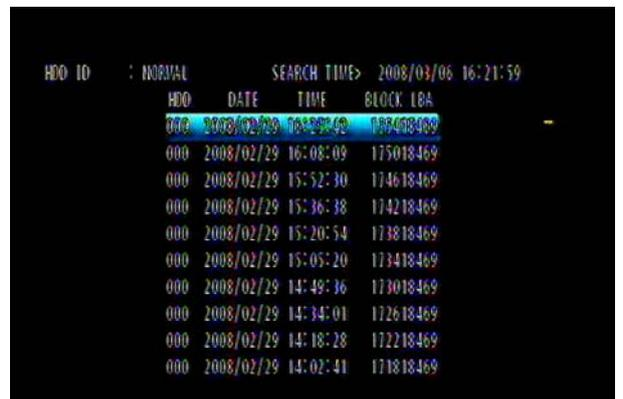
Select the desired HDD ID, TIME, BLOCK and press the ENTER button, the search results will be shown.
