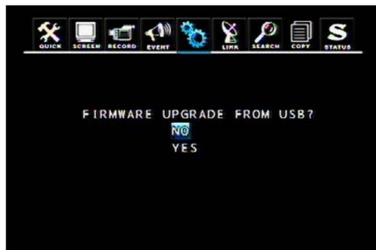
You can update the DVR firmware through the USB interface. Insert the USB device with the all.dvi file into DVR and press YES to update the firmware.
