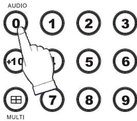
Audio ON/OFF: Press the FUNCTION button and then press the “AUDIO (0)” button to open/close the DVR audio function. You can hear audio of selected channel regardless of monitoring screen.
