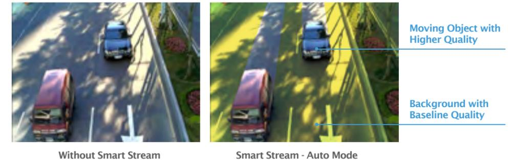
In this scenario, Smart Stream auto mode saves 30% of the original bandwidth required, while the detail of moving objects is maintained.
