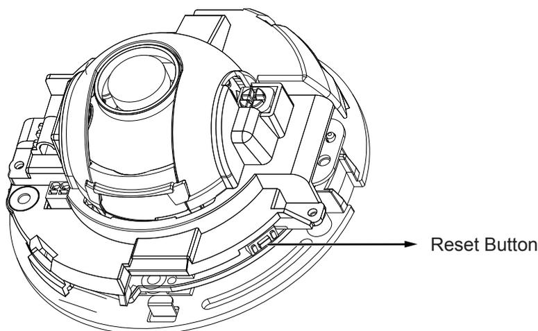
The reset button is used to reset the system or restore the factory default settings. Sometimes resetting the system can return the camera to normal operation. If the system problems remain after reset, restore the factory settings and install again.
