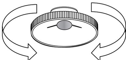
5. Use a piece of clean cotton cloth to hold and install the dome cover.
