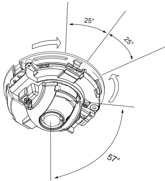
3. Tighten the camera's mounting screws after you change the horizontal shooting direction.
