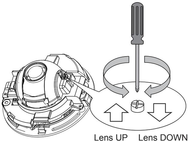
1. There is a tilt adjustment screw near the lens module. Use a #0, #1, or #2 Phillips screwdriver to turn the screw and the lens will move upwards or downwards.
