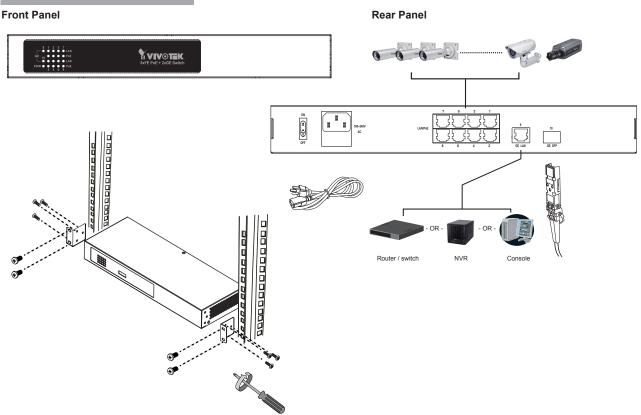
Use SFP, LC type transceiver with 100Mbps or 1Gbps transfer speed in Single mode (10km,30km,50km,80km) or Multi mode (0.5m or 2km) or Bidi (10km,30km,50km,80km).
