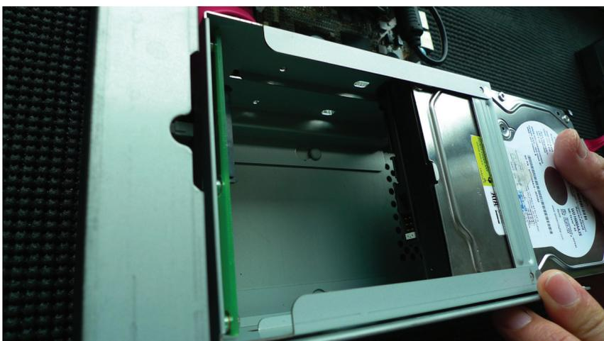
Make sure the SATA connectors are aligned with each other correctly
