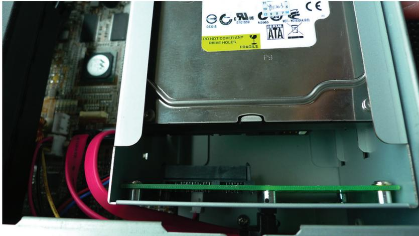
Secure the hard drive with the tool-less screw provided in the box
