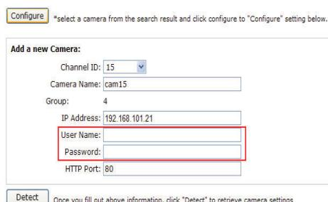
5. Click on "Detect" to establish connection between the recorder and the camera. If connection establishes successfully, camera's detailed information should be polled and displayed as below
