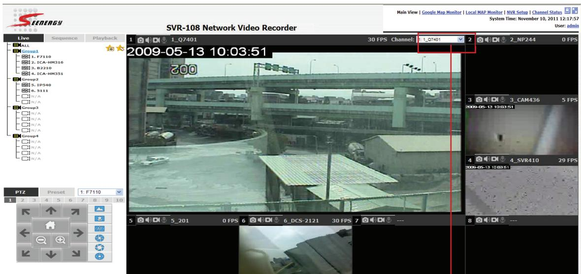
The 8 channel NVR comes with a 8-video split window view with one video displays on a larger window. Select a channel from the drop-down menu to display its video on the larger split window. You can also double-click on any of the smaller one to display its video to the larger window.
