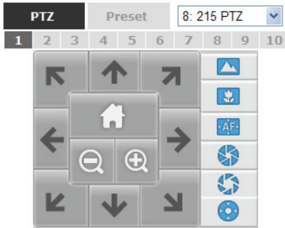
Camera(s) that are currently being selected for live viewing will be listed in the PTZ drop-down menu. Simply select a camera then use the PTZ control panel to control the camera
