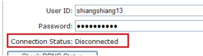
The NVR will automatically check with the DynDNS server once every hour and update its latest public IP to the server. The "Apply" button does the same thing which if you are see the "Disconnected" status, you can use it to manually check with the server without waiting for the NVR to update itself in the next hour. **However, it is advised not to do so too often as DynDNS disallow repetitive updates within a short period of time and the account will be banned if such action is detected.**
