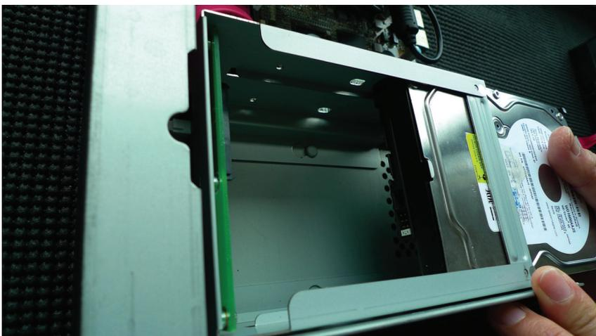
Make sure the SATA connectors are correctly aligned with each other.
