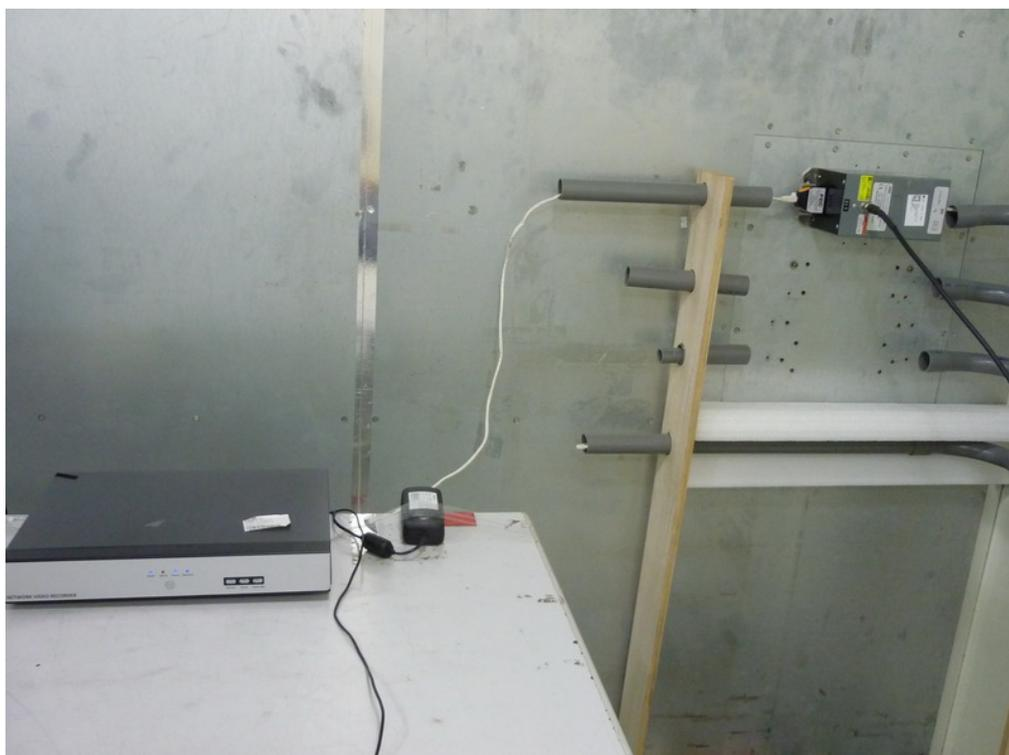
**Radiated Disturbance (Below 1GHz)****FULL SYSTEM D-SUB+HDMI 1920\*1080/60Hz(RECORD)**
