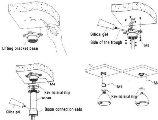
**Note: If the camera used in outdoor, Waterproof seal should be in the camera and bracket connecting part.**
