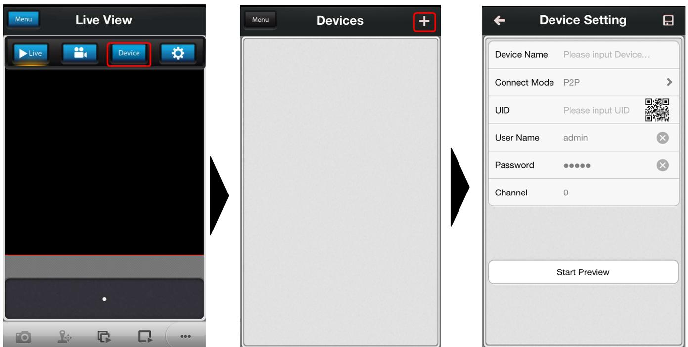
In the Device Setting screen, enter the details for your DVR/NVR/IPCam using the following as a guide:
