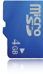
4 GB MicroSD card preinstalled in the camera (Q24M-Secure)
