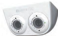
The difference between a MOBOTIX day-and-night camera and the standard versions is primarily that the MOBOTIX camera continuously uses two sensor modules rather than relying on a mechanical filter switch. In low light conditions, the hardware ensures an inherently better image quality, as a true infrared black-and-white image sensor is used instead of the usual color sensor with electronic color fade-out.
