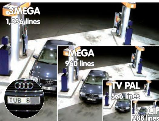
Original MOBOTIX camera image: Standard CIF compared to MOBOTIX HiRes
