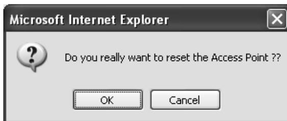
Click "OK" to reset the access point, or click "Cancel" to abort. Remember, all connections between wireless clients and this access point will be disconnected.
