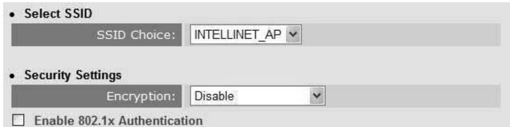
The screenshot shows a configuration window with two main sections. The first section, titled "Select SSID", contains a dropdown menu labeled "SSID Choice:" with "INTELLINET\_AP" selected. The second section, titled "Security Settings", contains a dropdown menu labeled "Encryption:" with "Disable" selected. Below these sections is a checkbox labeled "Enable 802.1x Authentication" which is currently unchecked.
