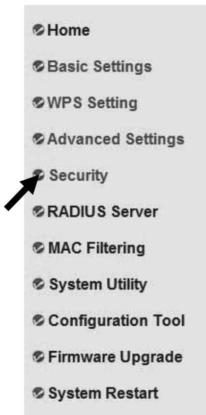
2. Click Set Security when the wireless operating mode you selected is AP Bridge-Point to Point, AP Bridge-Point to Multi-Point or AP Bridge-WDS.
