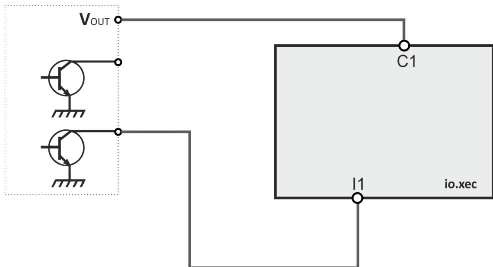
Please note that the activation voltage has no fixed polarization, therefore the terminal C1 can be connected to a positive or negative voltage.
