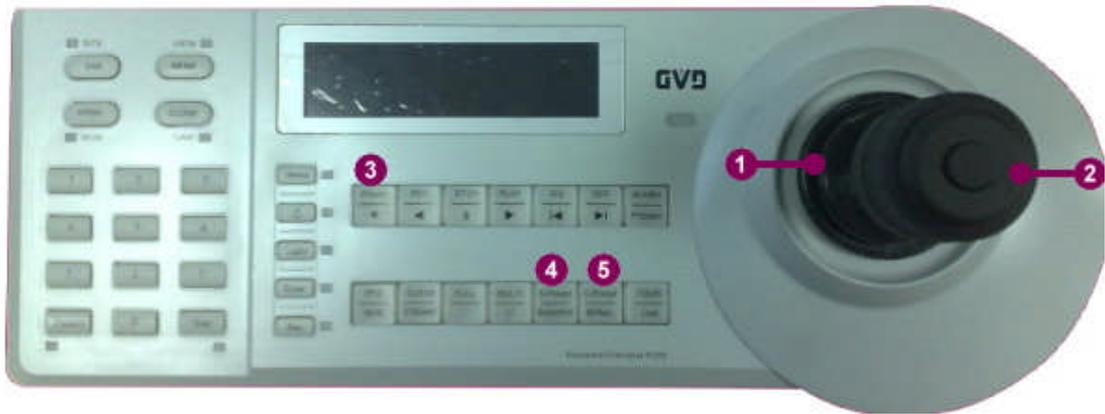
Figure 5-3 Function keys of PTZ mode
