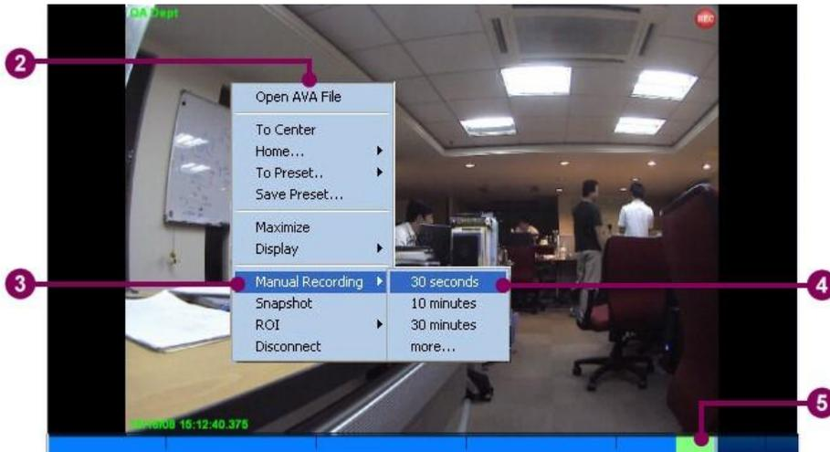
Figure 4-39 Manual Recording
