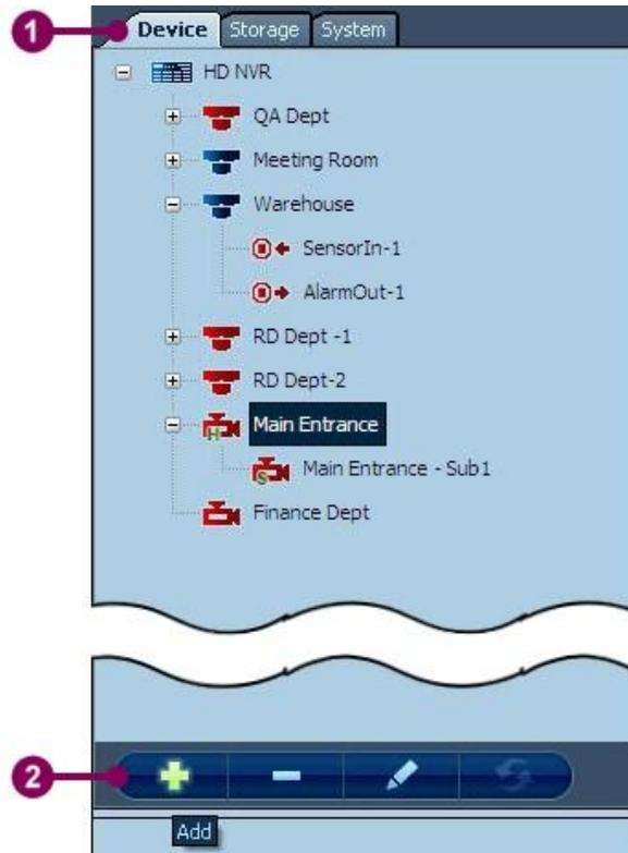
Figure 6-8 Add a channel automatically
