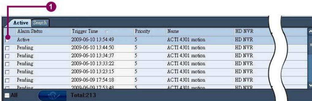
Figure 5-4 Acknowledge an alarm
