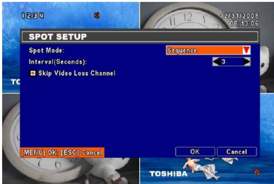
The DVR has two modes of video output; one is main video output, the other is spot video output. SPOT setup is for controlling the order of channels the system cycles through in SPOT mode. User can monitor every channel in the SPOT mode.
