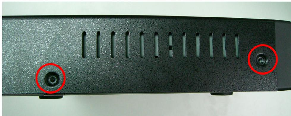
2. **Take off the cover. Place the HDD on the HDD rack and plug SATA connection.**
