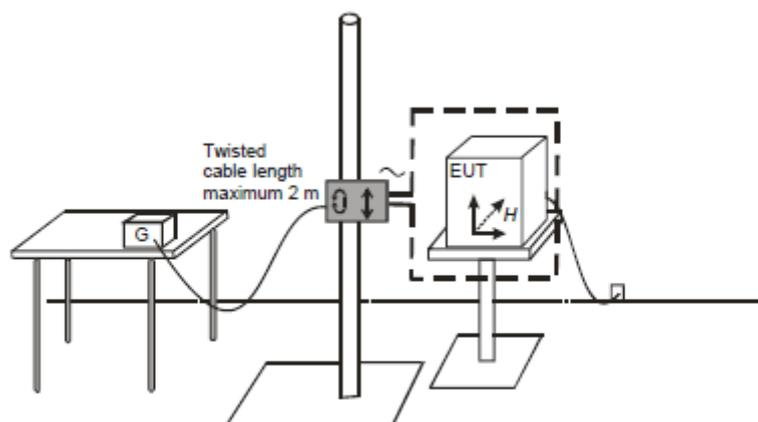
EUT : Equipment under test    G : Test Generator
