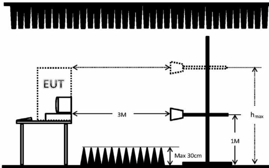
Remark: When EUT's height is over 172cm,  $h_{max}$  = top of EUT
