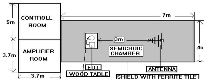
**NOTE : The SPORTON 7m x 4m x 4m semi-anechoic chamber is compliance with the sixteen point's uniform field requirement as stated in IEC 1000-4-3 Section 6.2.**
