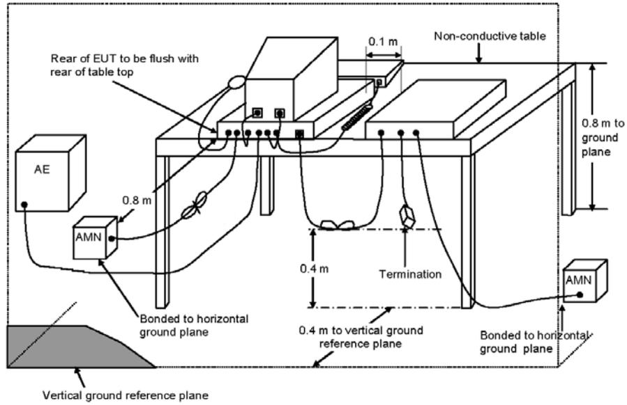
**5.4. Typical Test Setup Layout of disturbances at telecommunication ports**
